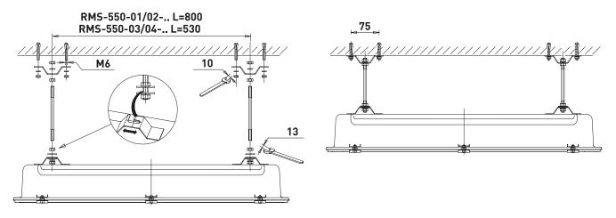
Note: Expansion bolts (for concrete) or bolts (for steel frame) are not included in our kit.
