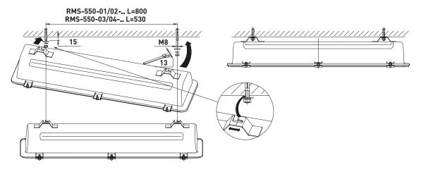
Note: Expansion bolts (for concrete) or bolts (for steel frame) are not included in our kit.
